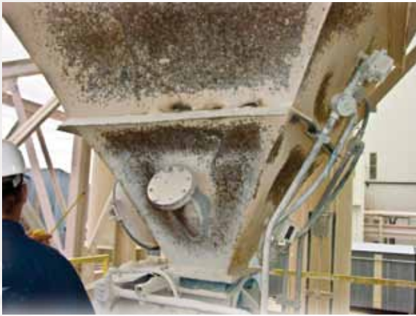
Hammering on the bin or chute wall leads to damage to the wall surface, often called "hammer rash."
