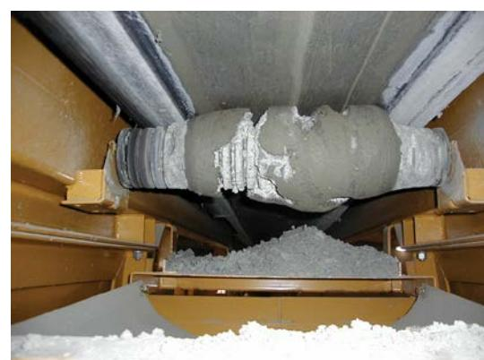
*Carryback can build up on idlers, causing issues with mistracking.*
