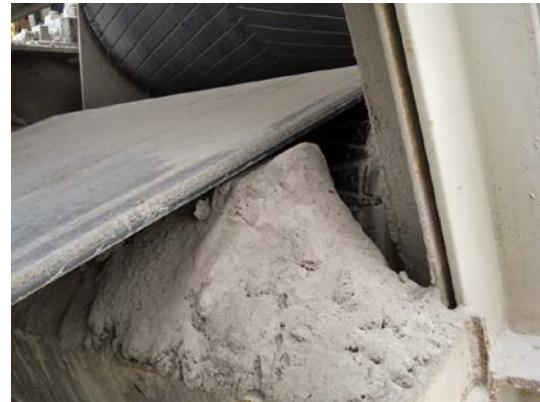
*Removed from the belt, carryback can attach to other surfaces, including the belt-cleaning system and the vertical walls of the chute.*
