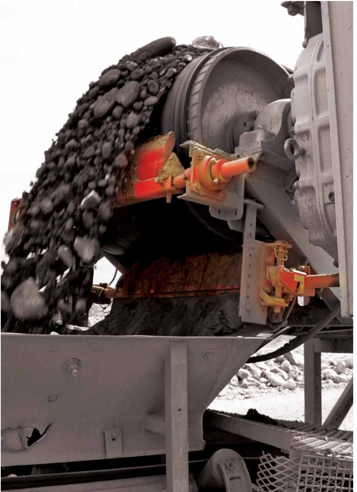
▲ Martin Belt Cleaners remove carryback from conveyors carrying run-of-mine ore or finished concentrate.
